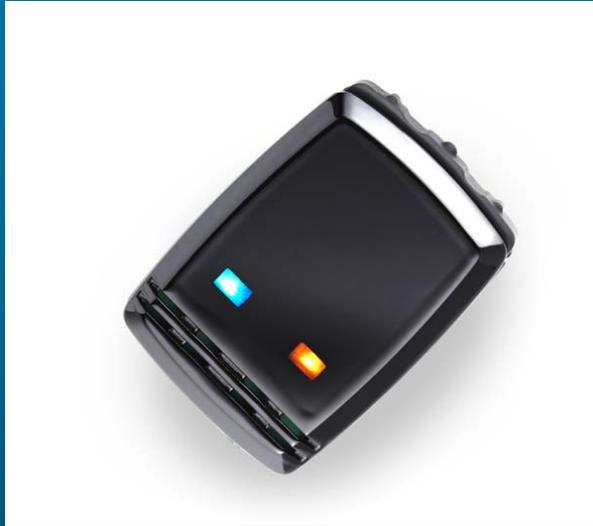
Visual and audible indicators provide sound processor status and low battery warning
