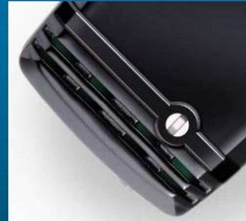
The optional tamper-proof door keeps the battery from being removed
